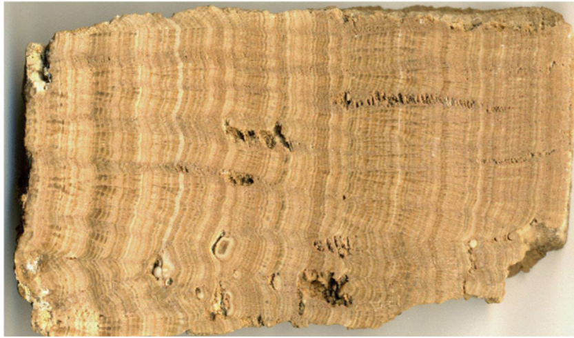
10 cm thick carbonate deposits from the Roman aqueduct of Cologne, Germany, representing 180 years of deposits.
